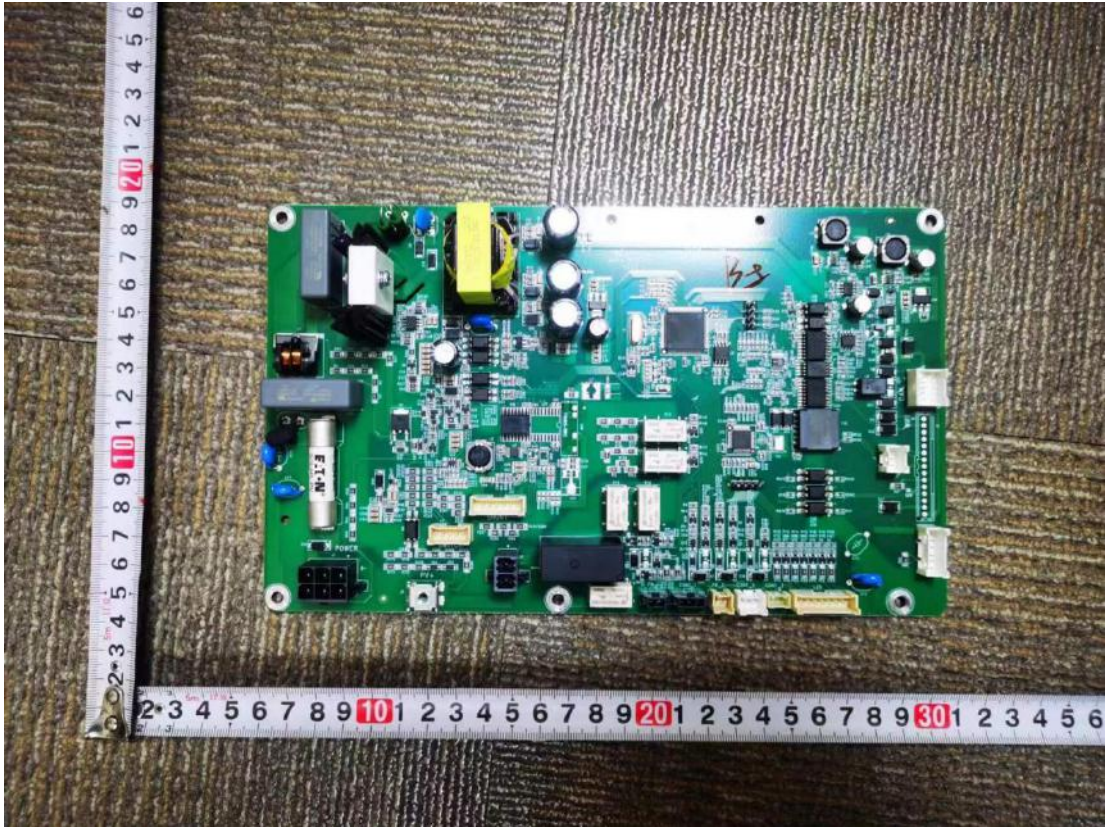
Main control board in Main control unit (Top view)
